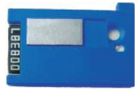
TLD card type RADOS with 0,5mm Al-filter
